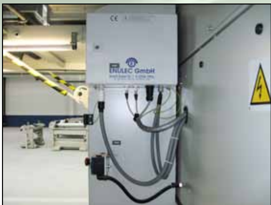
ESA 1000 Capacitance Free Power Supply integrated into a new rotogravure press
