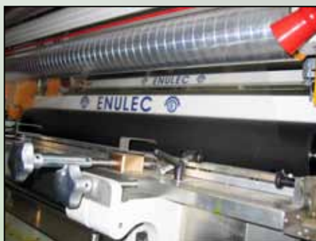
Enulec ESA 1000 Dot Skip Eliminator with integrated static eliminators on entry and exit of print station.
