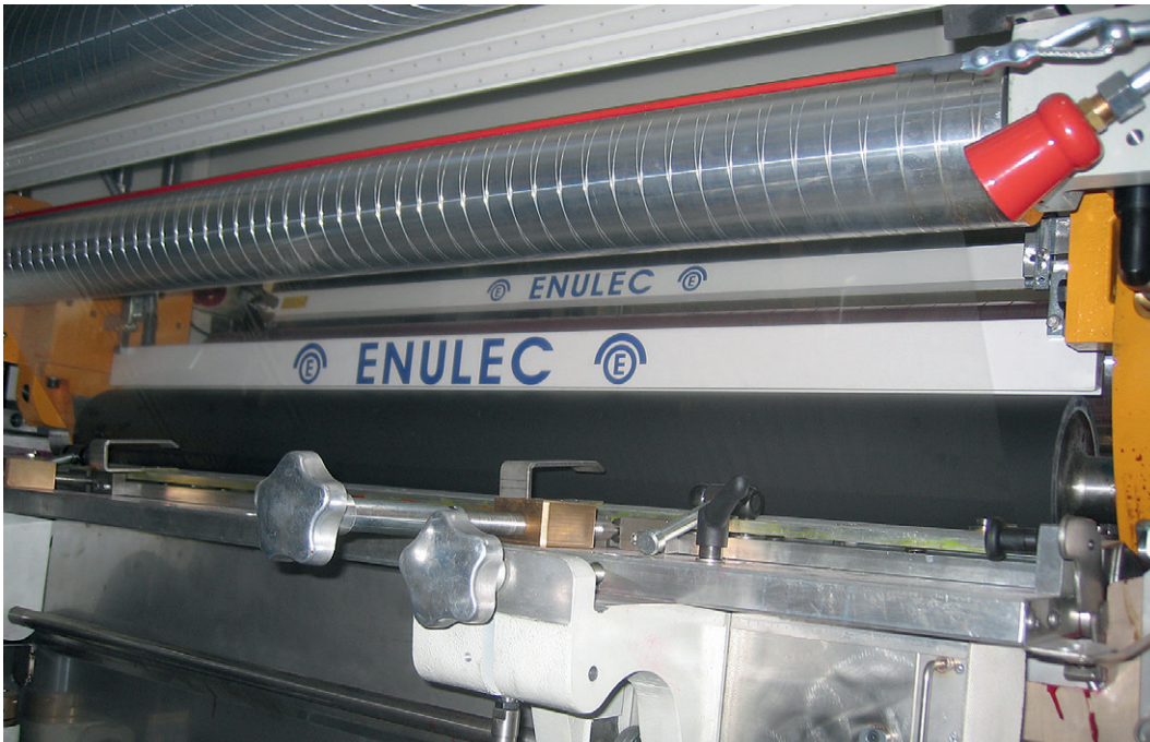
An ESA system in a gravure printing station
